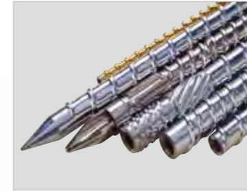
Special plasticizing components Special high efficiency high mixing chrome screw for PET preform, in order to ensure low shear condition to achieve high efficiency and high quality plasticization, improve shrinkage problems, improve transparency.
