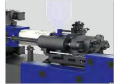
linear guide rails are used for injection movement High rigidity injection unit, low friction coefficient, high operation precision, low energy consumption.
