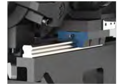
Linear guide rails are used for injection movement High rigidity injection unit, low friction coefficient, high operation precision, low energy consumption.
