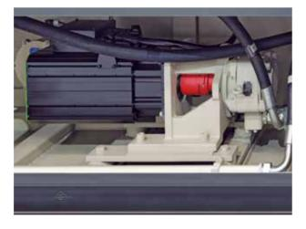
The new servo motor with low inertia is equipped with high speed hydraulic pump to provide better acceleration response performance. It provides stable and reliable hydraulic driving force for injection, opening and closing mold and other actions. The perfect combination of economy and performance.
